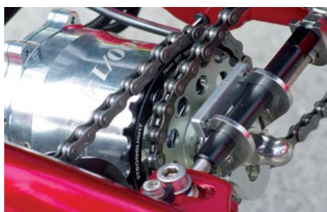
(Above) The boom and chain guides provide lots of adjustment for rider height
