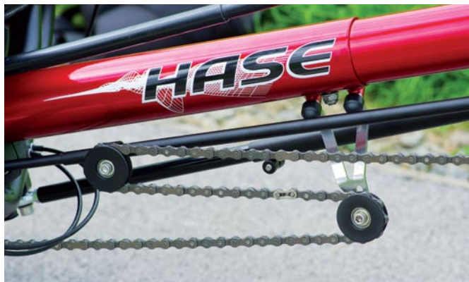
(Above) The boom and chain guides provide lots of adjustment for rider height
