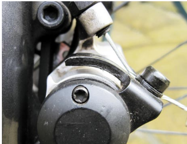
This disc calliper has been incorrectly adjusted. The cable should be in contact with the cam
