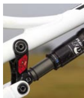
There's less room – or requirement – for suspension with bigger wheels. This Trek has 110mm
