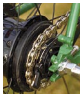
(Above) Shimano's 11-speed Alfine hub gives a 409% range (Top) It's also available in 1x10 and singlespeed versions, with different frames
