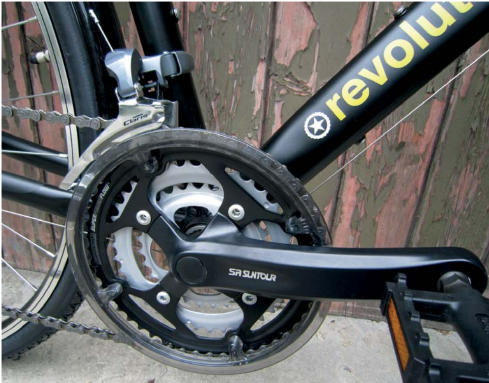
Left: Some tourers come with road triples. Both of these have a trekking triple with 28-38-48 chainrings, giving a small reduction in gearing that's nevertheless worth having when carrying luggage
