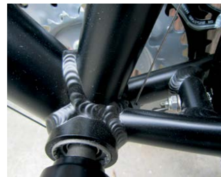
Above: Both bikes feature inexpensive square-taper bottom brackets, which will likely last longer than comparable external bearing units
