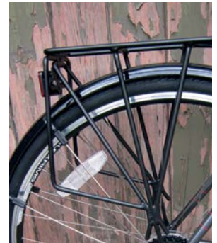
■ The Ridgeback, like the Revolution, is equipped with the touring essentials: mudguards and a rear rack. Either can be fitted with a low-rider front rack
