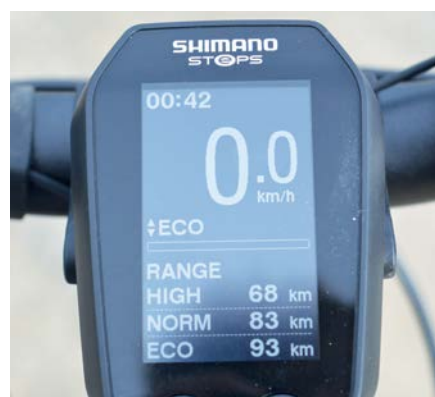
Above: The head unit shows how much juice you've got left in different modes, but the figures are estimates only
